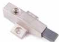
Hinge side carcass mounted BLUMOTION, to suit all straight arm hinges with 0mm raised mounting plate BLUM971A0500
