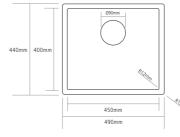
Min. base unit 500mm For cut-out shape go to www.caple.co.uk for template
