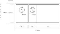
Main bowl depth 200mm Small bowl depth 150mm Min. base unit 600mm Cut-out size 990 x 420mm
