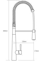
Worktop cut out 35mm required Note: Pull-out hose extended by 600mm → DIMENSIONS
