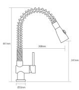
Worktop cut out 35mm required Note: Pull-out hose extended by 410mm
