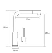
Worktop cut out 35mm required Note: Pull-out hose extended by 660mm
