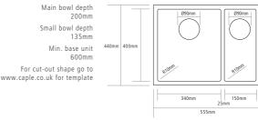
Small bowl depth 135mm For cut-out shape go to www.caple.co.uk for template STAINLESS STEEL
