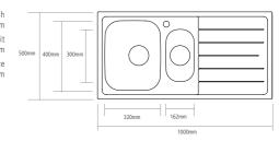
Main bowl depth 200mm Small bowl depth 128mm Min. base unit 600mm Cut-out size 978 x 480mm
