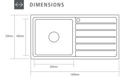
Bowl depth 200mm Min. base unit 600mm Cut-out size 980 x 480mm
