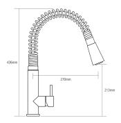
Worktop cut out 35mm required Note: Pull-out hose extended by 600mm
