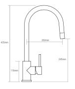
Worktop cut out 35mm required Note: Pull-out hose extended by 500mm
