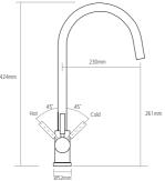
Worktop cut out 35mm required Note: Pull-out hose extended by 650mm
