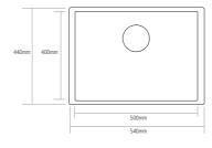
Bowl depth 200mm Min. base unit 600mm Inset cut-out size 420 x 520mm Undermount cut-out size 405 x 505mm
