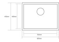
Bowl depth Min. base unit Cut-out size 550 x 400mm For cut-out shape go to www.caple.co.uk for template
