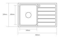
Main bowl depth 200mm Min. base unit 450mm Cut-out size 780 x 480mm
