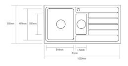
Main bowl depth 200mm Small bowl depth 175mm Min. base unit Cut-out size
