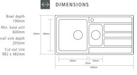
Main bowl depth 190mm Small bowl depth 110mm Min. base unit 600mm Overall sink depth 205mm Cut-out size 982 x 482mm
