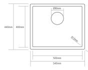
Bowl depth 200mm Min. base unit 600mm For cut-out shape go to www.caple.co.uk for template
