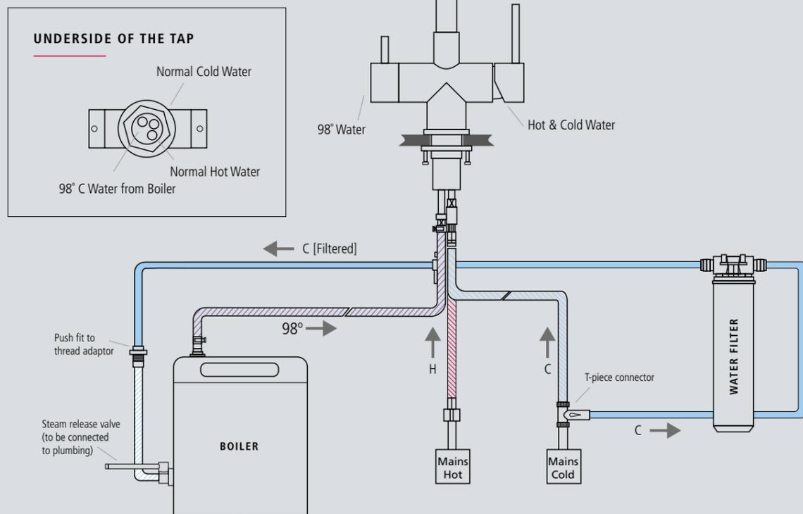
Diagram above shows Vapos 3in1 steaming hot water tap.
